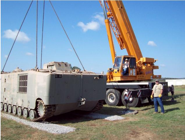
The orange thing in the picture is a 100 ton crane. It places the 35 ton LVTP-5A1 gently into position near the Visitor Center (see picture on back page). The LVTP is a Landing Vehicle Tracked Personnel and it was used in Vietnam exclusively by Marines. It has a Continental V-12 engine.
